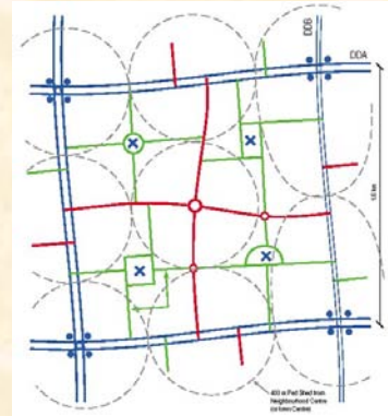
A 256 ha transportation Network model by the PCWA rests on the 400m rule.
